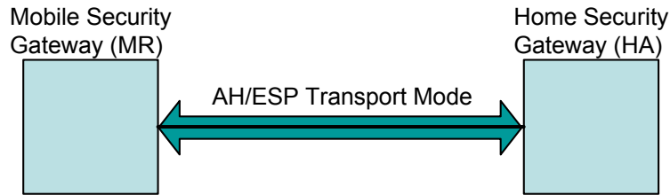
Figure 9: IPsec protection of BU and BAcK
